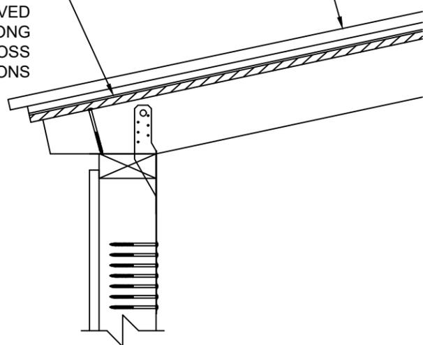
2 **METAL ROOF FASTENING DETAIL**
