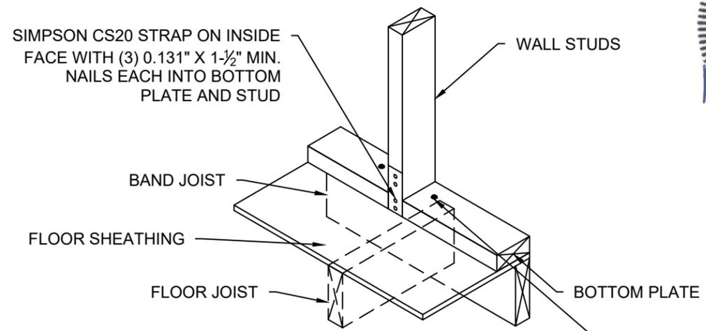
1/4" x 4" HEX LAG SCREWS WITHIN 3" ON EITHER SIDE OF STUD AT X-BRACE END LOCATIONS AND CENTERED THRU BAND JOIST - (2) SCREWS IN SIDE WALL AND END WALL WITHOUT OPENINGS, AND (4) SCREWS IN END WALL WITH OPENINGS SPACED MIN. 1" APART. PREDRILL MAX. 1/4" DIA. HOLE THRU BOTTOM PLATE AND 0.15" DIA. HOLE THRU SHEATHING AND BAND JOIST.
