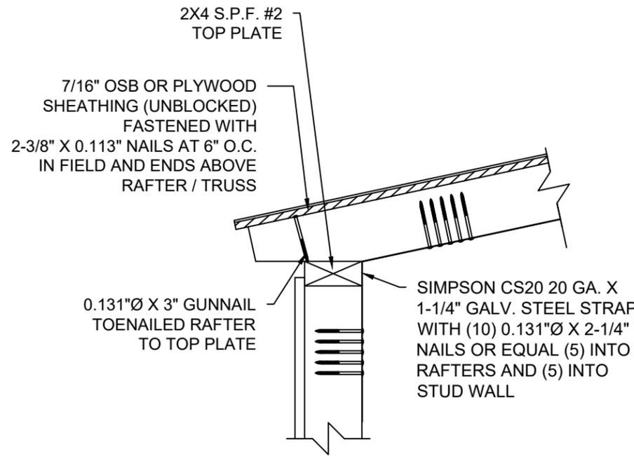
5 **ALTERNATE WALL STUD TO RAFTER DETAIL**
