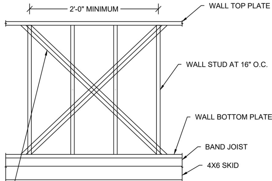
(2) SIMPSON CS18 (43MIL X 1-1/4", GRADE 40 STEEL, G60 COATING) X-STRAP OR EQUIVALENT ON INSIDE FACE OF WALL STUD. ATTACH STRAPS TO WALL TOP & BOTTOM PLATES WITH 0.131" x 2-1/4" NAILS STAGGERED - (4) NAILS IN SIDE WALL, (6) NAILS IN END WALL WITHOUT OPENINGS AND (10) NAILS IN END WALL WITH OPENINGS. STRAP MAY BE WRAPPED AROUND WALL TOP & BOTTOM PLATES.
