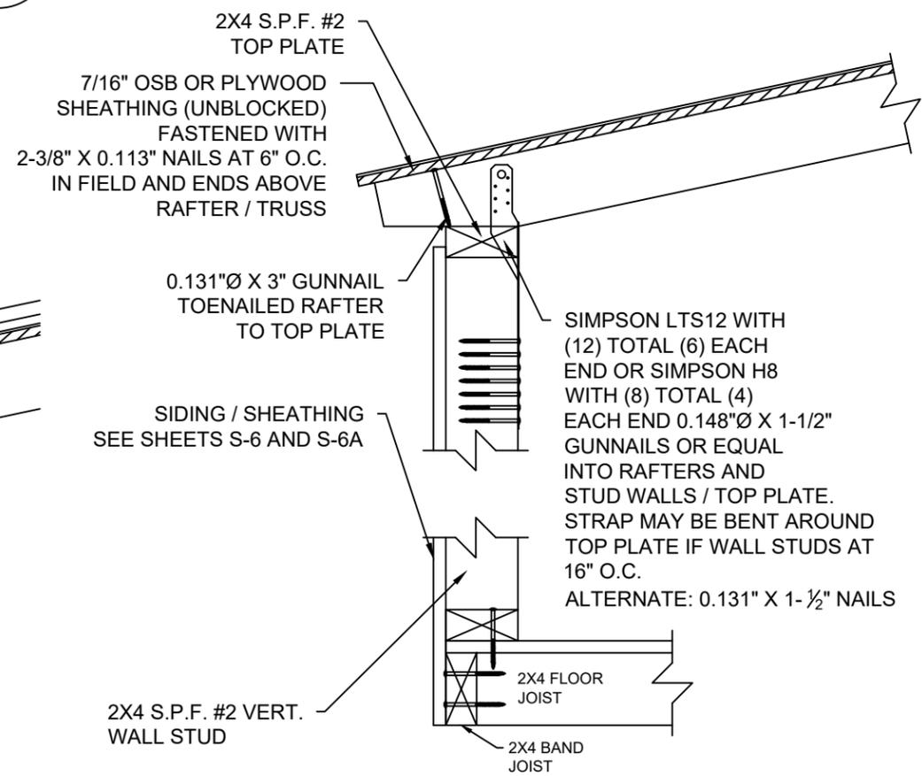
3 **WALL STUD TO RAFTER / TRUSS AND FLOOR FASTENING DETAIL**
