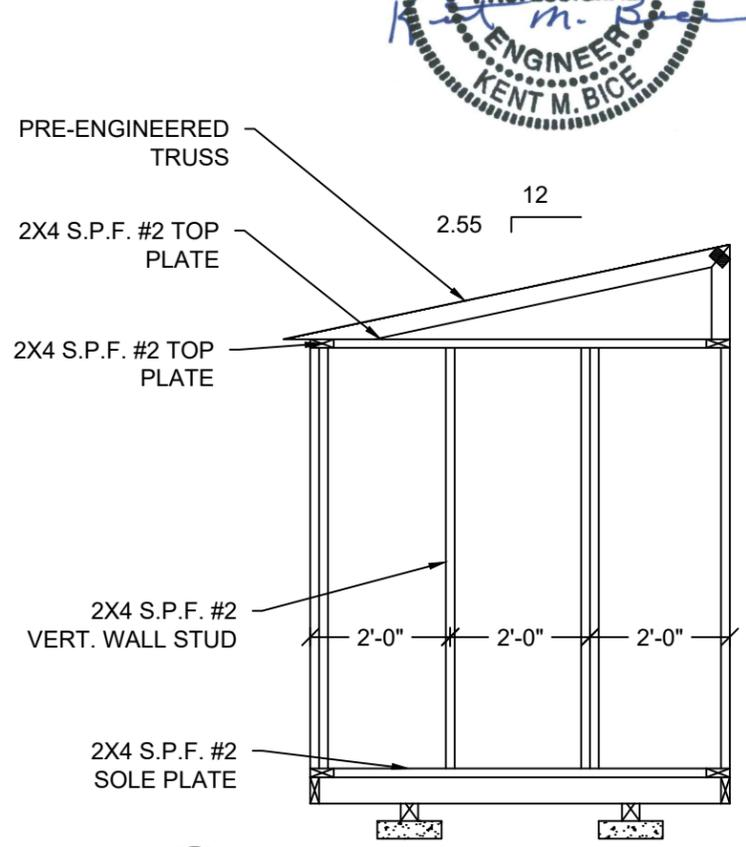
**3 ENDWALL FRAMING ELEVATION**
