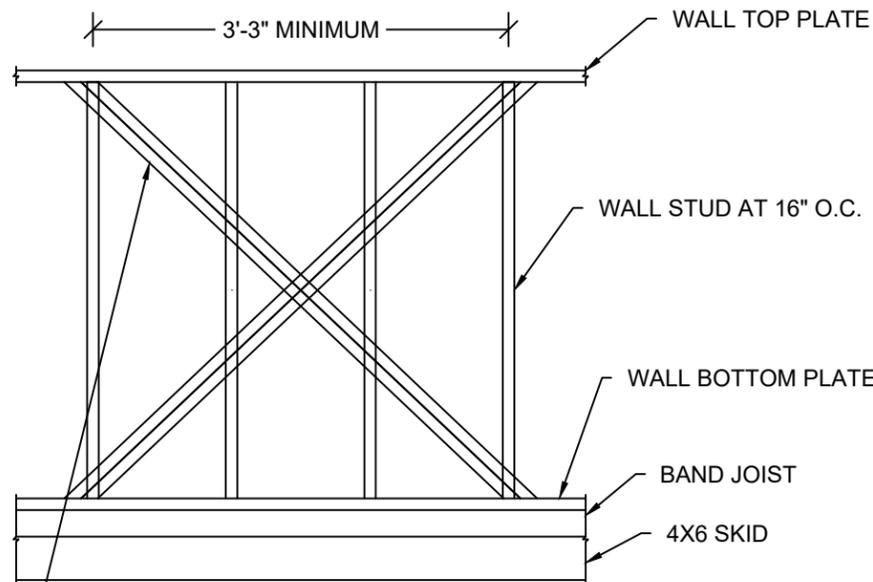
(2) SIMPSON CS20 (33MIL X 1-1/4", GRADE 40 STEEL, G60 COATING) X-STRAP OR EQUIVALENT ON INSIDE FACE OF WALL STUD. ATTACH STRAPS TO WALL TOP & BOTTOM PLATES WITH (5) 0.131" x 2-1/4" NAILS STAGGERED. STRAP MAY BE WRAPPED AROUND WALL TOP & BOTTOM PLATES.
