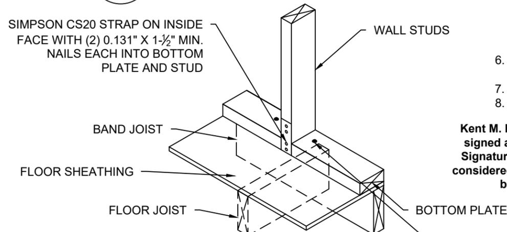
(2) 1/4" x 4" HEX LAG SCREWS WITHIN 3" ON EITHER SIDE OF STUD AT X-BRACE END LOCATIONS AND CENTERED THRU BAND JOIST. PREDRILL MAX. 1/4" DIA. HOLE THRU BOTTOM PLATE AND 0.15" DIA. HOLE THRU SHEATHING AND BAND JOIST.
